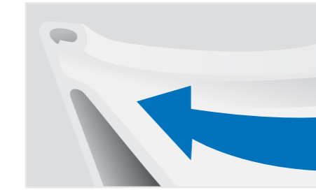
All water flows out from the top of the bowl, cleaning the inner surface of the bowl.
