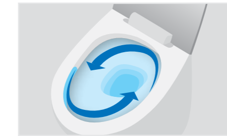
100% of the water is ejected through two water openings.
